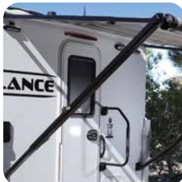
Rear Awning. The awning can be either pull-out or electric, depending on the specific model. Shade your door and rear your camper.
