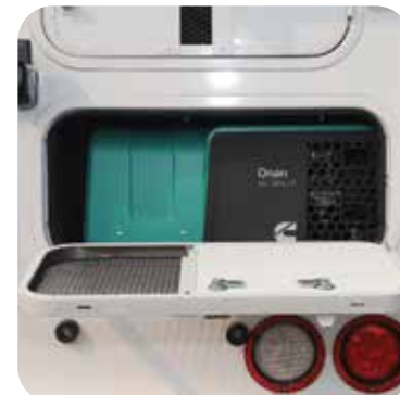
Generator: 2500 Watt LPG (Onan). This propane generator provides true off-grid independence and functionality for all systems. Available on select models
