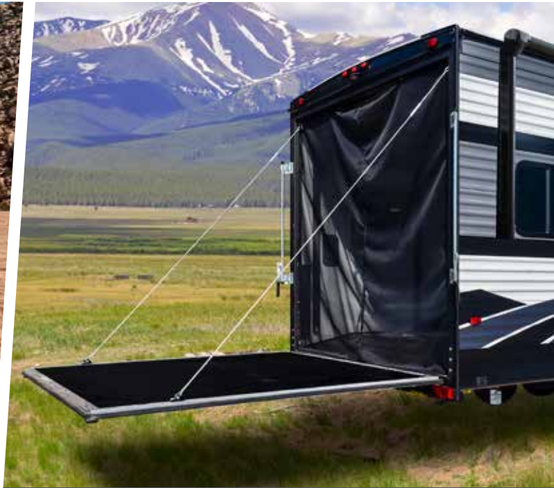
True wide body design to fit all stock side by sides. Featuring 6 tie downs, more than any other brand to safely secure your toys up to 5000 lbs.
